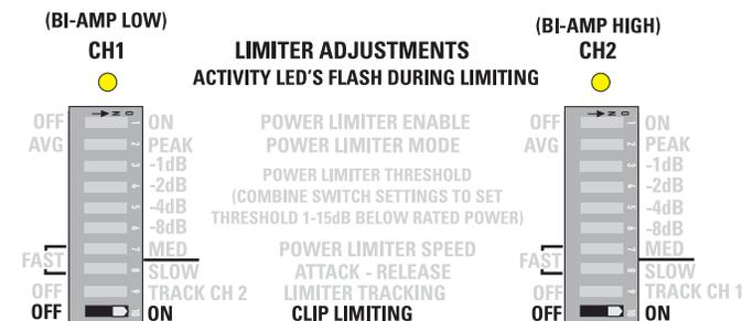
FOR STEREO TRACKING: ENABLE BOTH LIMITER TRACKING SWITCHES.
