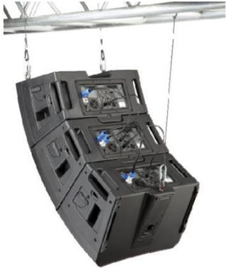
KLA offers solutions for both permanent and temporary suspension. For permanent installations each element has four M10-threaded points on the top of the cabinet, and one in the bottom center of the rear of the cabinet for aiming.
