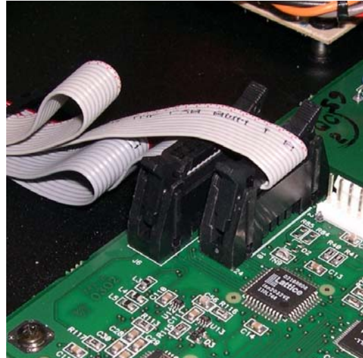
Figure 3. Reconnecting the header.
