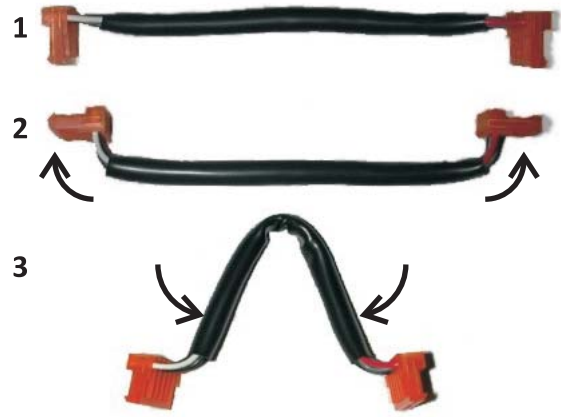
Figure 3. Preparing the cable: 1. Starting point. 2. Bend cable 90 degrees at the ends so the housings point straight out. 3. Bend the middle of the cable as shown.
