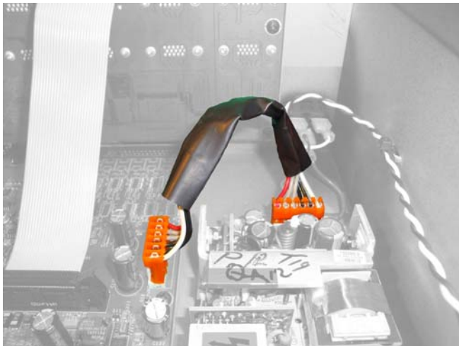
Figure 4. The new power supply interface cable, installed.
